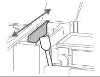
Use the cleaning stick to remove the ink and dust on the circumference of the cap.
