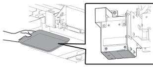
Use a paper towel to clean dust or ink off the underside of the UV-LED lamp.
